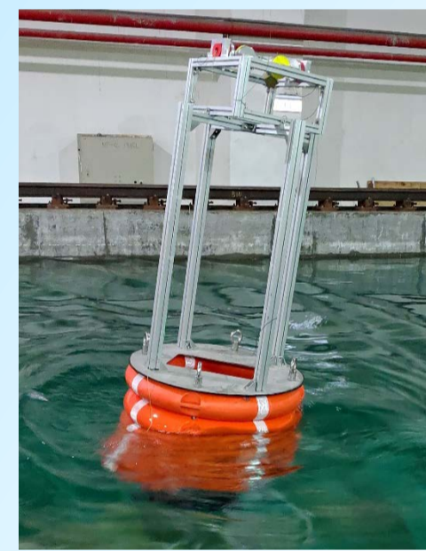
Enhancement of rolling energy conversion of buoys using eccentric rotors. PZT energy harvester for tire pressure sensor.
