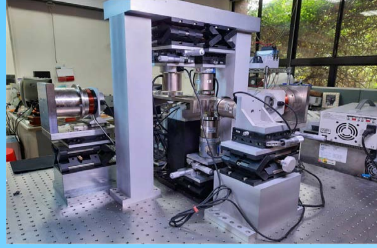
6 and 4-axis force/torque sensors design, Calibration machine
